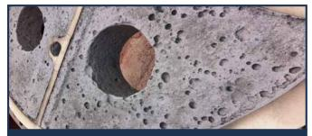
Channel in cooing water, pitted surface blasted clean exposing many pits deeper than 0.0625"
