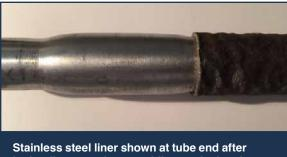
hydraulic expansion, providing a tube in tube repair to corroded exchanger tube.
