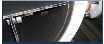
New fabrication heat exchanger channel, ID coated with Curran 1500, applied to 0.040" in a single coat.
